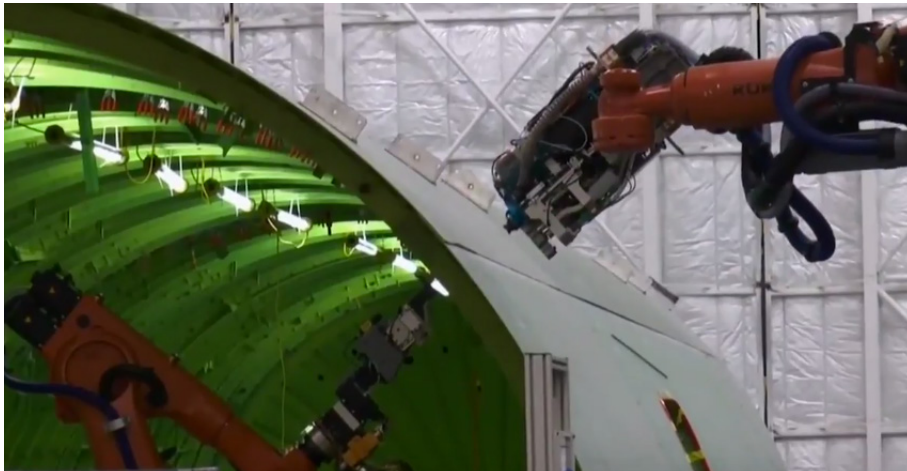
Robotic drilling systems used in the production of civilian aircraft fuselage.
