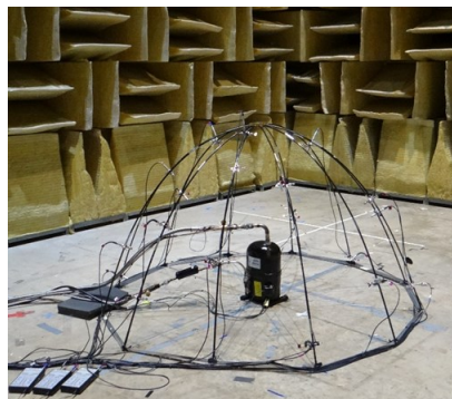
A Bristol compressor in ARL/Penn State's hemi-anechoic chamber
