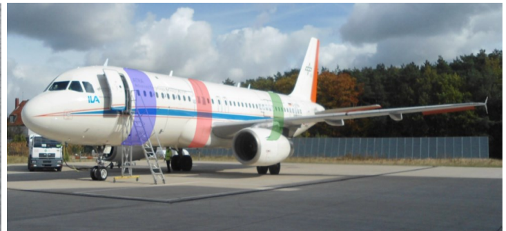
Figure 2. Surface pressure measurements on vehicles: Top – underwater towed body with internal hydrophone array from Bundeswehr Technical Center, Germany; Bottom – instrumented aircraft (colored regions indicated high sensor density) from DLR, Germany.
