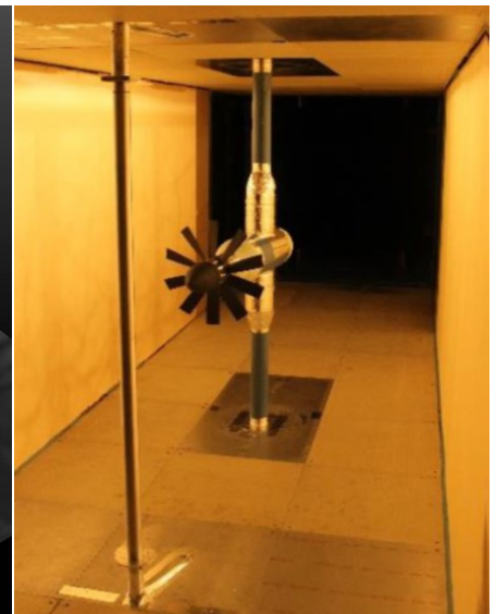
Figure 1. Left - Pratt and Whitney simulation of supersonic jet discharge flow over a downstream structural panel; Right - measurement of turbomachinery noise in Virginia Tech wind tunnel
