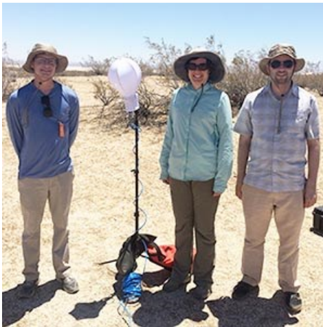
Summer 2016 novel sonic boom measurements in the Mojave Desert near NASA's Armstrong Flight Research Center. Left to right: Will Doebler (Acoustics Ph.D. Candidate), Eigenmike 32 element spherical microphone array with white wind screen, Michelle Vigeant (Assistant Professor of Acoustics and Architectural Engineering), Trevor Stout (Acoustics Ph.D. Candidate). Image provided by Will Doebler.
