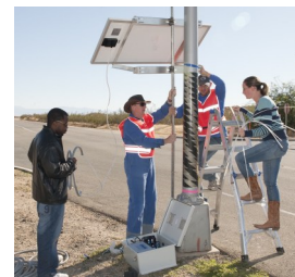
Fig. 2. NASA Dryden WSPR project principal investigator Larry Clatt, Wyle's Christopher Hobbs, Gulfstream's Joseph Salamone (wearing the Penn State ball cap) and NASA Dryden engineer Erin Waggoner install one of 13 remote sonic boom sensors. The sensors were placed throughout the Edwards AFB residential community to remotely measure sonic
