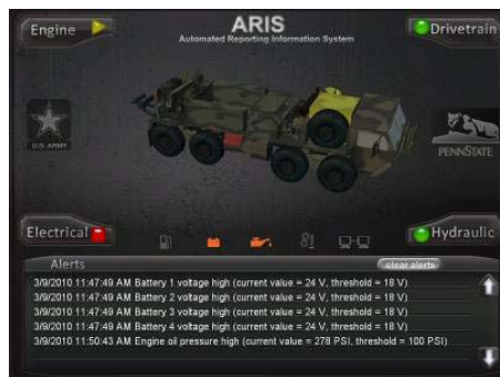
Figure 4 Top-level display showing 3-D representation of platform with color-coded alert and alarm messages,
