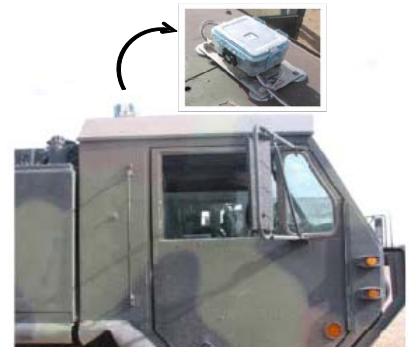
Figure 6 Collision avoidance warning system
