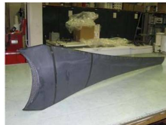
Figure 2 Prototype composite wind turbine blade – a 3-axis accelerometer will be mounted inside each blade monitoring unsteady loads
