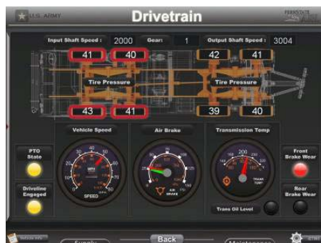
Figure 5 System schematic with critical health and status information
