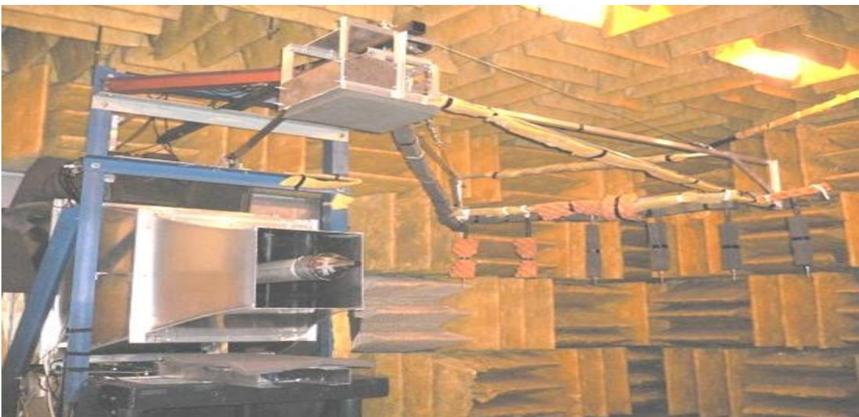
The jet plenum and forward flight duct installed in the anechoic chamber.
