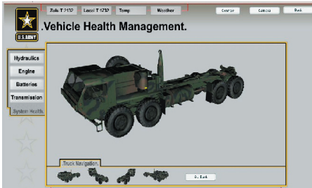
Figure 1 - HEMTT health monitoring system user interface.
